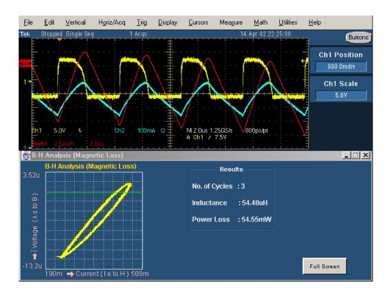
TDSPWR2 Power Analysis Measurements Reference
